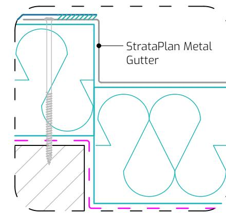
Timber batten mechanically fixed to decking
