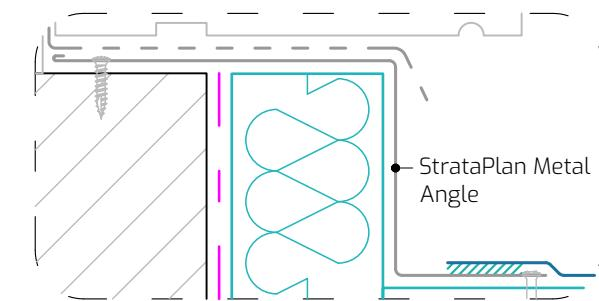
Sill projecting min. 45mm with a min 30mm drip away from the face of the upstand.
