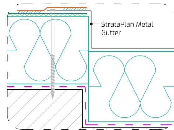
Timber batten mechanically fixed to decking
