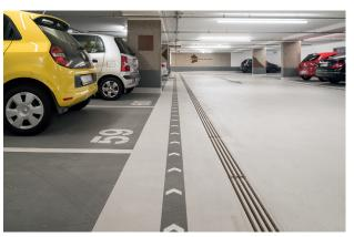
The driving lanes were given a light, reflective finish. Parking bays and arrow markings were offset in dark grey.
